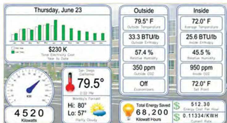
FIGURE 2 Level 1 dashboards typically display facility energy performance data streamed from energy meters and the building automation system.
